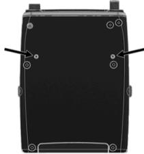
Using one included L-hex key, remove the set screws on the back of the A20-TX transmitter, if present.
